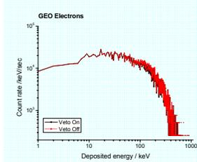
Electron spectra – deposited energy - at GEO orbit with and without veto counter
