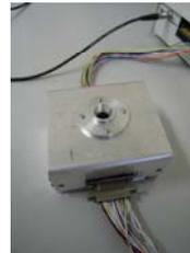
LEED laboratory model for tests with  $\gamma$  and e<sup>-</sup> sources
