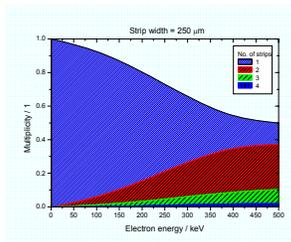
Number of strips responding to single electron vs. initial energy (W=250  $\mu$ m)
