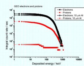
Proton and electron integral spectra with and without Al-absorber at GEO orbit
