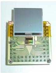
Si microstrip and readout chip on the test-board
