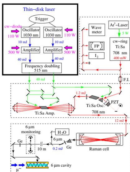
An experiment using a new ultra-low energy muon beam (bottom) and a dedicated  $\lambda = 6 \mu\text{m}$  laser system (left) was set up at PSI, and first data were taken in Nov. 2003. The statistics were too low to determine the  $2S - 2P$  resonance line. Next data taking is planned for 2007, with a thin-disk laser developed at IFSW Stuttgart, enhancing the event rate by a factor 20.
